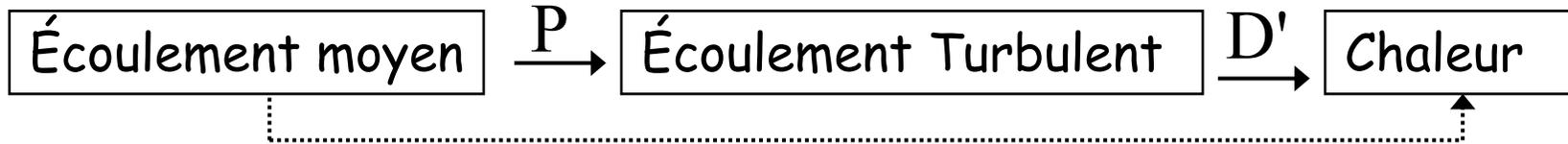
$$\underbrace{\frac{1}{\rho} F_j \langle \bar{u}_j \rangle_f}_{\text{Puissance dissipée}} = \underbrace{\frac{\nu}{V_f} \int_{V_f} \left( \frac{\partial \bar{u}_i}{\partial x_j} \right)^2 dV}_{\text{Chaleur}} - \underbrace{\left\langle \overline{u'_i u'_j} \frac{\partial \bar{u}_i}{\partial x_j} \right\rangle_f}_{\text{Turbulence } \bar{P}}$$
