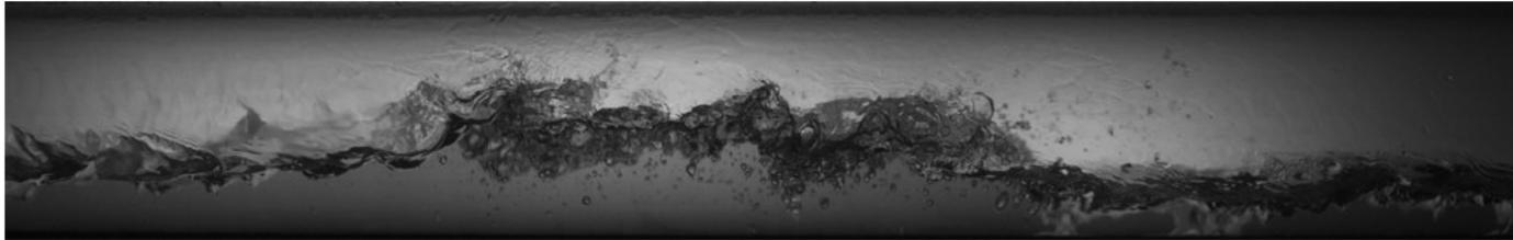
Photo 17, Wavy-stratified flow, with roll waves, Test 33
