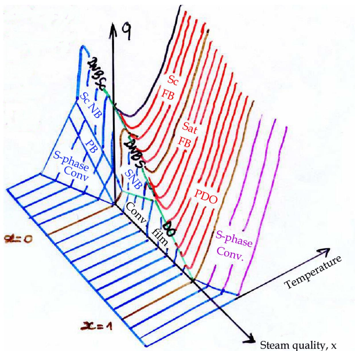
S-Phase conv: single-phase convection, PB: partial boiling, NB: nucleate boiling (S, saturated, Sc, subcooled), FB: film boiling, PDO: post dry-out, DO: dry-out, DNB: departure from nucleate boiling.
