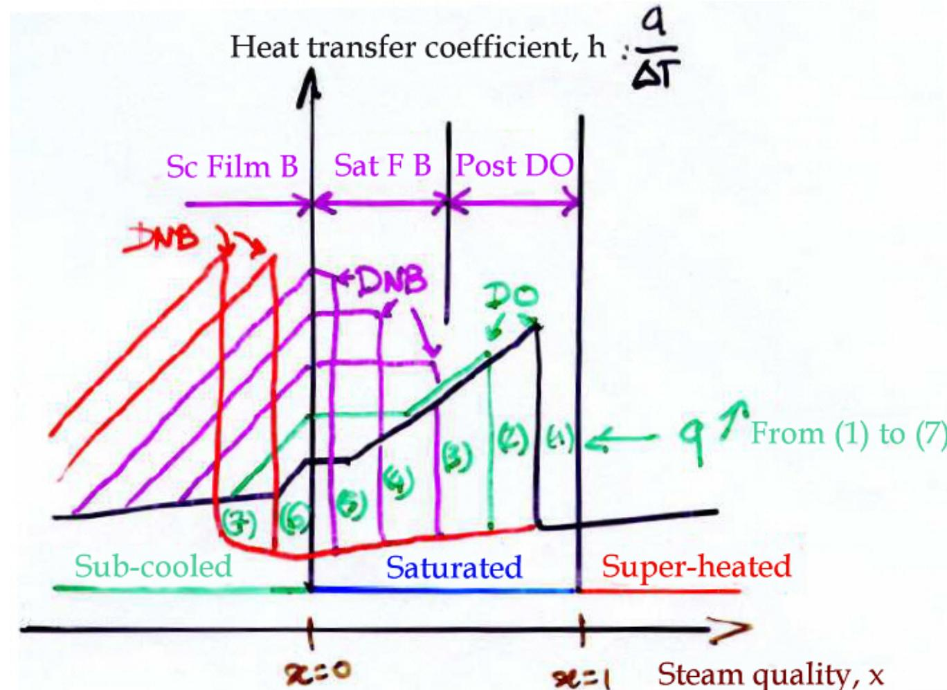
DO: dry-out, DNB: departure from nucleate boiling (saturated, sub-cooled), PDO: post dry-out, sat FB: saturated film boiling, Sc Film B: sub-cooled film boiling
