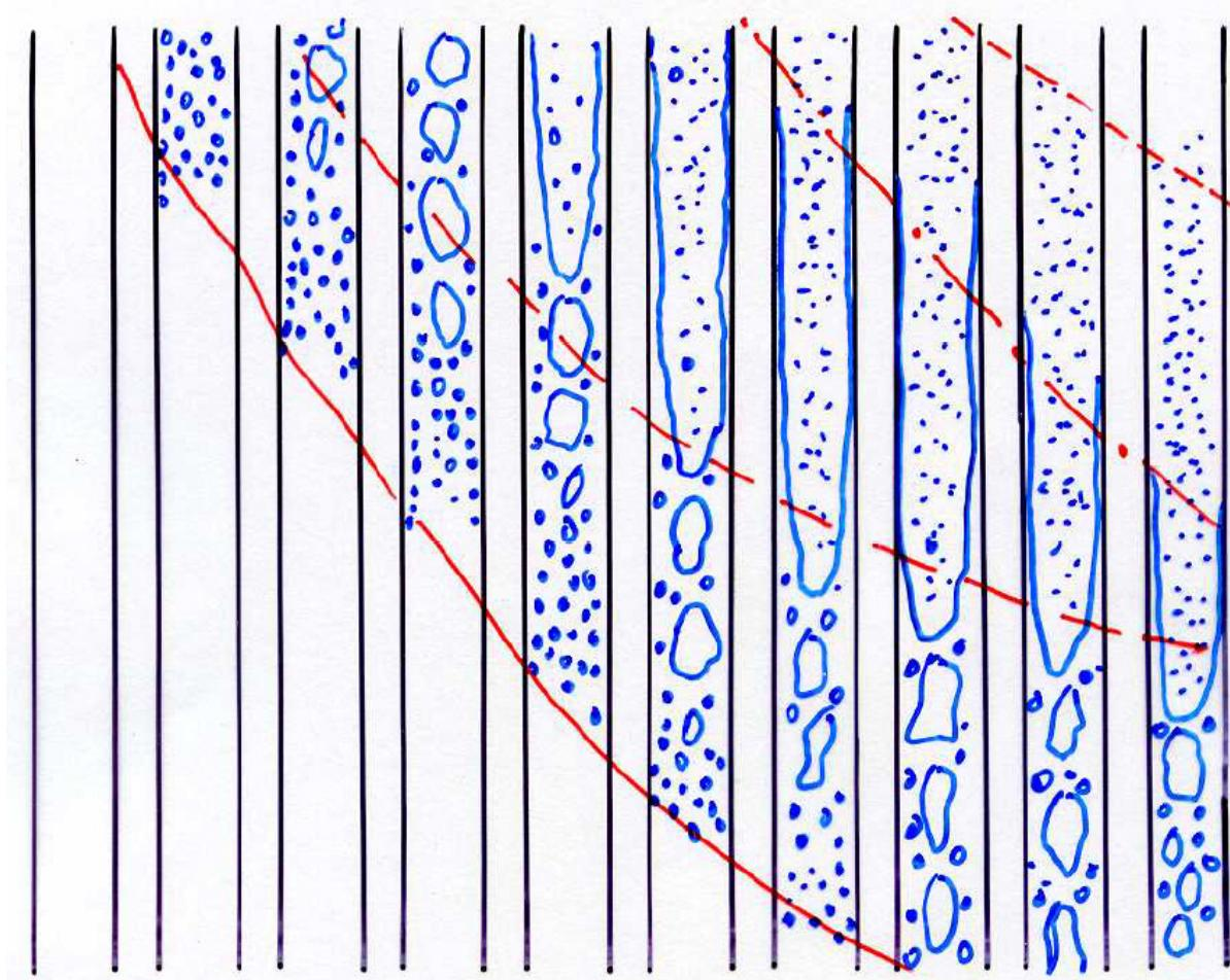
→ Increasing heat flux, constant flow rate →
